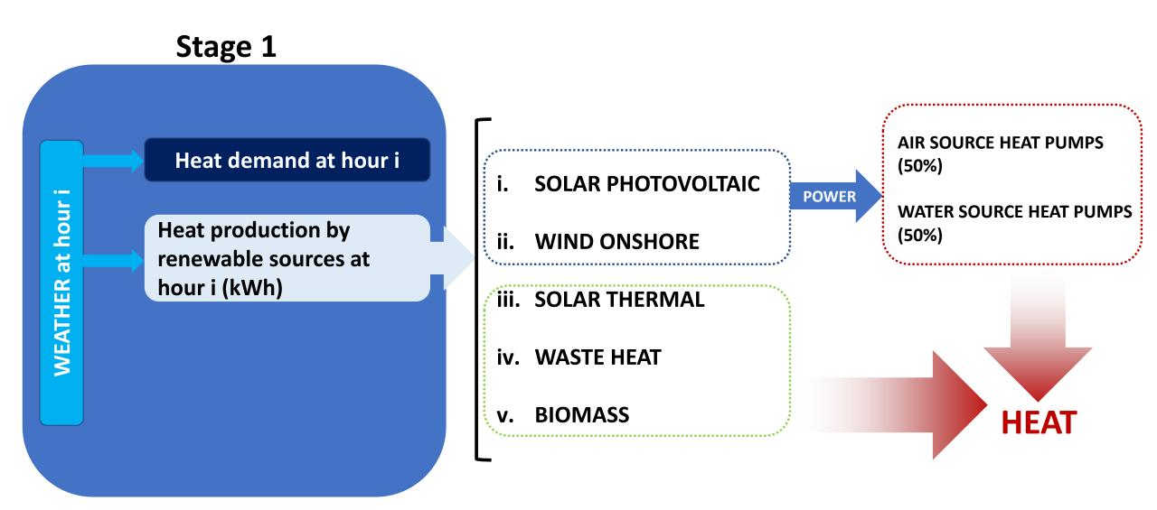
Heat output produced by heat pumps powered by SPV and Wind turbines
