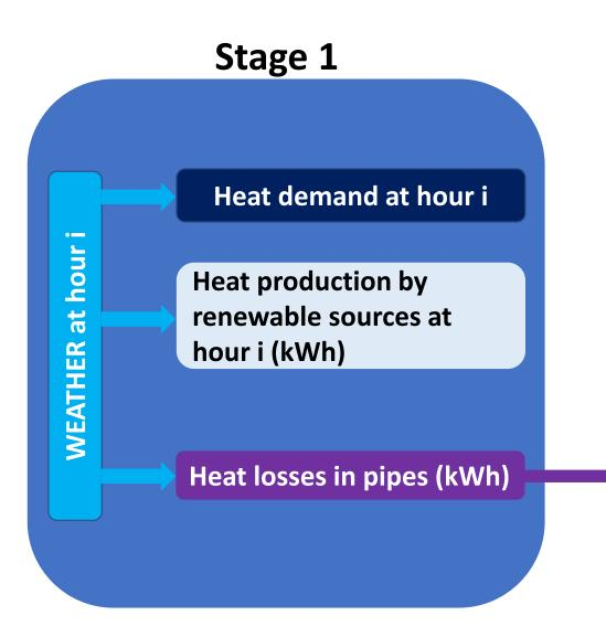
$$HL_{p,x \text{ to } y,i} = 2 \cdot \pi \cdot \lambda \cdot L_{x \text{ to } y} \cdot \frac{\left(T_{in} - T_{out,i}\right)}{ln\left(\frac{r_{out}}{r_{in}}\right)}$$
