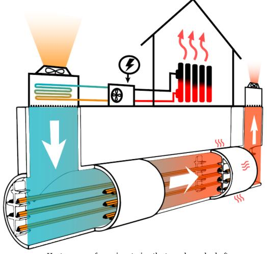
Heat recovery from air entering the tunnel supply shaft: reduced tunnel air temperature and cable losses
