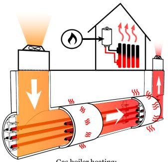
Gas boiler heating: high tunnel air temperature and high power cable losses
